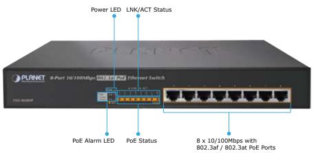
All RJ-45 copper interfaces in the FSD-808HP support 10/100Mbps Auto-Negotiation for optimal speed detection through RJ-45 Category 6, 5 or 5e cables. It also supports standard Auto-MDI/MDI-X that can detect the type of connection to any Ethernet device without requiring special straight or crossover cables.
