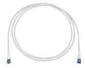
Cable identification: S/FTP Outer jacket: LSFRZH Conductor diameter copper strand: AWG 26/7 Screened in pairs: AL/foil Overall screen: copper braid Outer diameter: max. 6.2 mm
